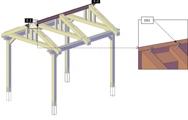
**Step 11:** Use 5/16" x 6" lag bolts (**LB3**) to attach the rafters (**8**) to the ridge beam (**7**) and to the supports with 3" deck screws (**DS2**). Check the marked on each rafter and place as drawings shown.
