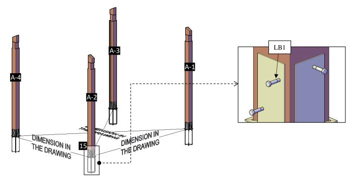
**Step 2:** Use 3/8" X 7 ½" bolts (**BL1**) with washer and nuts to attach the single supports (**2**) to the posts. Check the marked on each support and place as drawings shown.
