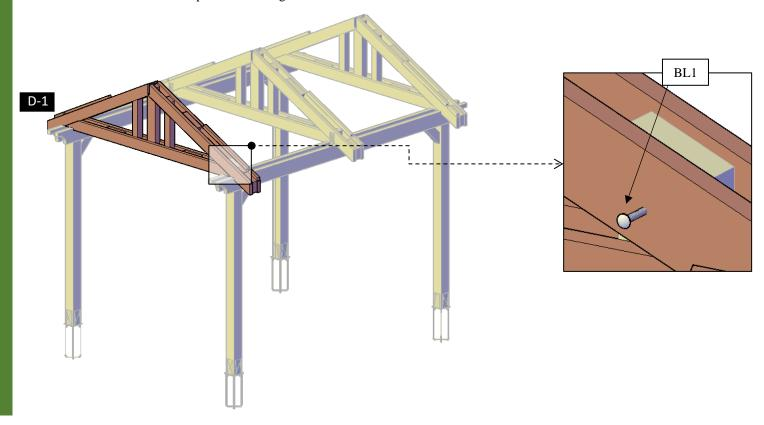
**Step 9:** Attach the Secondary knee braces (6) to the roof trusses (4) with 3/8" X 7  $\frac{1}{2}$ " bolts (**BL1**) with washer and nuts and to the posts with 3/8" x 9" bolts (**BL2**). Check the marked on each secondary knee brace and place as drawings shown.
