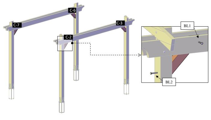
Step 5: Attach the metal plaques (14) to the supports with 3/8" x 3" lag bolts (LB2).
