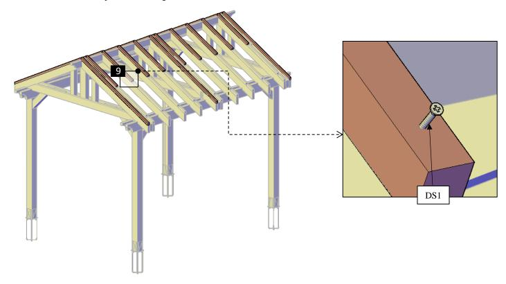
Step 13: Attach the rafter reinforcement (10) to the rafters (8) with 2<sup>---</sup> deck screws (DS2). Check the marked on each rafter reinforcement and place as drawings shown.
