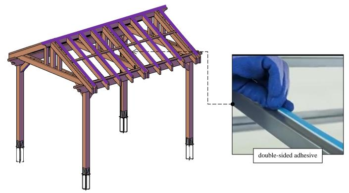
**Step 16:** use 2" deck screws (**DS3**) with neoprene washers to attach the polycarbonate (**12**) to the rafter. After that, attach the Profile-H and Profile - H click to the rafters and to the ridge beam (**12**) with 2" deck screws (**DS3**). Check the marked numbers on each polycarbonate and place as drawings shown.
