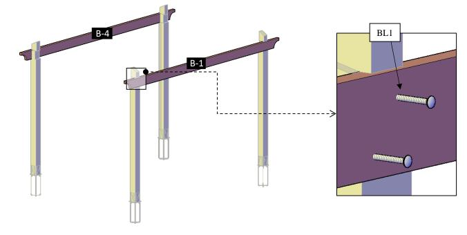
**Step 3:** Attach the single supports to the supports with in-between blocking (3), use 3/8" X 7 ½" bolts (**BL1**) with washer and nuts. After that, return to the bolts described in the step 3 and tighten fully. Check the marked on each support with in-between blocking and place as drawings shown.
