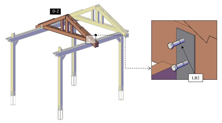
**Step 8:** Attach the perimeter Roof Trusses (4) to the posts with 3/8" X 7 <sup>1</sup>/<sub>2</sub>" bolts (**BL1**) with washer and nuts. Check the marked numbers on each roof truss and place as drawings shown.
