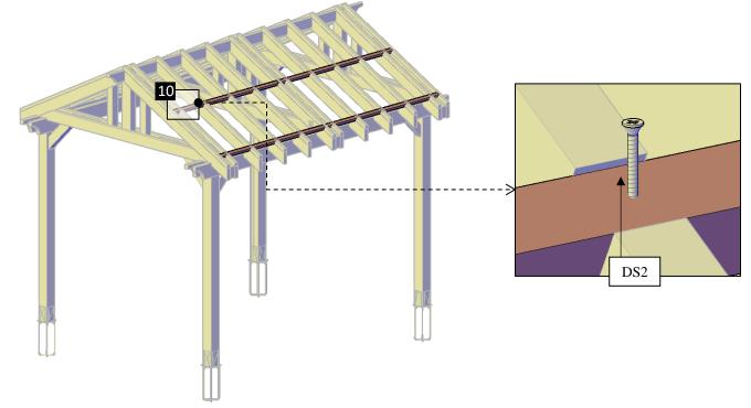
Step 14: Put metal tape 48mm x 50m on the polycarbonate exterior sides and the perforated tape on the interior side.
