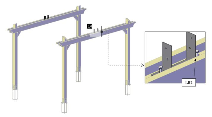
**Step 6:** Attach the perimeter Roof Trusses (4) to the posts with 3/8" X 7 <sup>1</sup>/<sub>2</sub>" bolts (**BL1**) with washer and nuts. Check the marked numbers on each roof truss and place as drawings shown.
