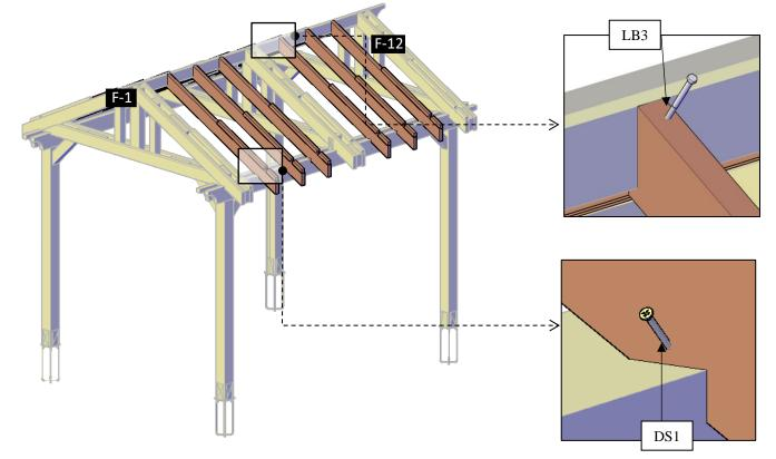
Step 12: Use 3" deck screws (DS1) to attach the increase rafter (9) to the rafter (8) and to the roof trusses (4). Check the marked on each increase rafter and place as drawings shown.
