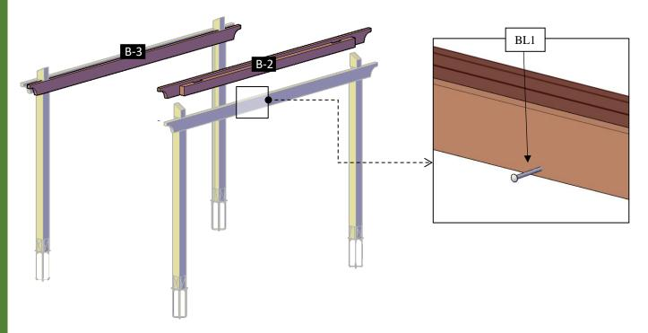
**Step 4:** Attach the main knee braces (5) to the supports with 3/8" X 7  $\frac{1}{2}$ " bolts (**BL1**) with washer and nuts and to the posts with 3/8" x 9" bolts (**BL2**). Check the marked on each main knee brace and place as drawings shown.
