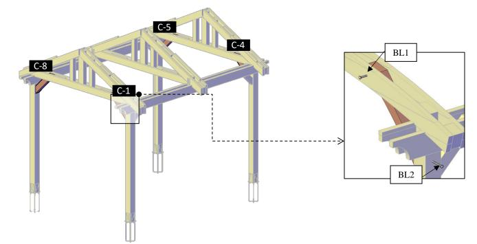
Step 10: Attach the ridge beam (7) to the roof trusses (4) with 3" deck screws (DS1). Check the marked on each ridge beam and place as drawings shown.
