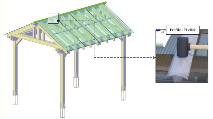
Step 18: Put exterior clear silicone on the polycarbonate joints.
