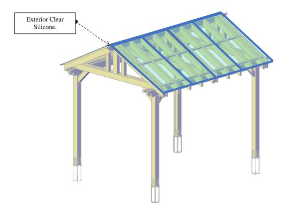
Step 19: Attach the fascias (16) to the rafters and roof trusses with 3" deck screws (DS1). Check the marked numbers on each fascia and place as drawings shown.
