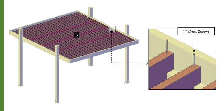
**Step 5:** Use 5/16" x 3" lag bolts (**B**) with washers (**K**) to attach the rafters (**4**) marked in red to the supports-A. Each part has a series of numbers that indicate where to attach the part with the corresponding number.
