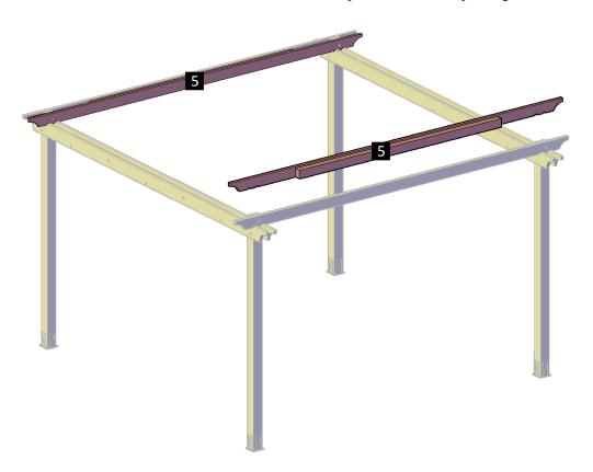
Step 7: Attach the single rafters to the rafters with in-between blocking (5), use 3/8" X 7" bolts (D).
