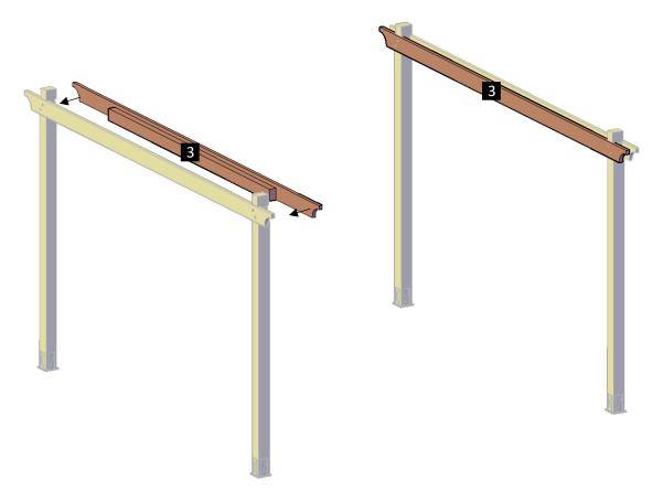
Step 4: Attach the single supports to the supports with in-between blocking (3), use 3/8" X 7" bolts (D).
