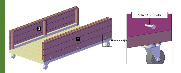
**Step 2:** Attach the short walls (3) to the long walls with 5/16" x 2" bolts (A), as shown below. Each part has a series of numbers that indicate where to attach the part with the corresponding number.
