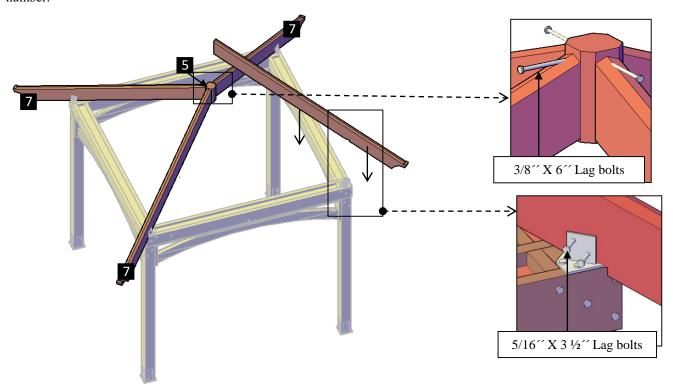
**Step 9:** Attach the central rafters (6) to the second frame (5) with 5/16 x 4 ' lag bolts (I) and to the single supports (2) with 3/8 x 10 lag bolts (D). Each part has a series of numbers that indicate where to attach the part with the corresponding number.
