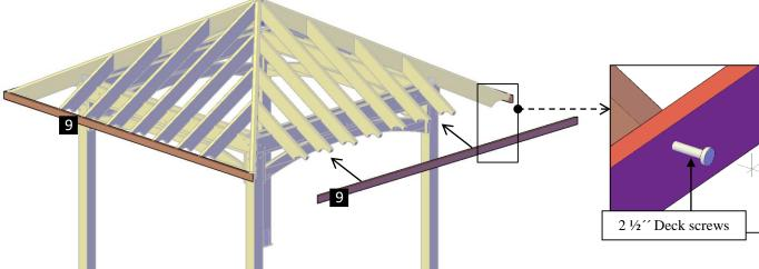
**Step 13:** Use 1.5/8" x 6" deck screws (**K**) to attach the roof boards (**10**) to the rafters, central rafters and diagonal rafters. Put the boards from the bottom to the top. Each part has a series of numbers that indicate where to attach the part with the corresponding number
