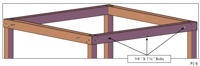
Step 5: Attach the arcs (4) to each post with 3/8" x 7" bolts (F).
