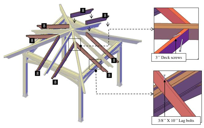
**Step 11:** Attach the rest rafters (8) to the diagonal rafters and to the single supports (2) with 3" deck screws (J). Each part has a series of numbers that indicate where to attach the part with the corresponding number.
