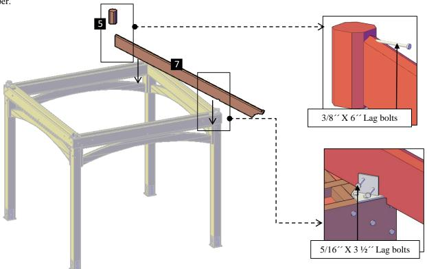
**Step 8:** Attach the rest diagonal rafters (7) to the second frame (5) with 3/8" x 6" lag bolts (C) and to the rest metal plaques (12) with 5/16" x 3 ½" bolts (H). Each part has a series of numbers that indicate where to attach the part with the corresponding number.
