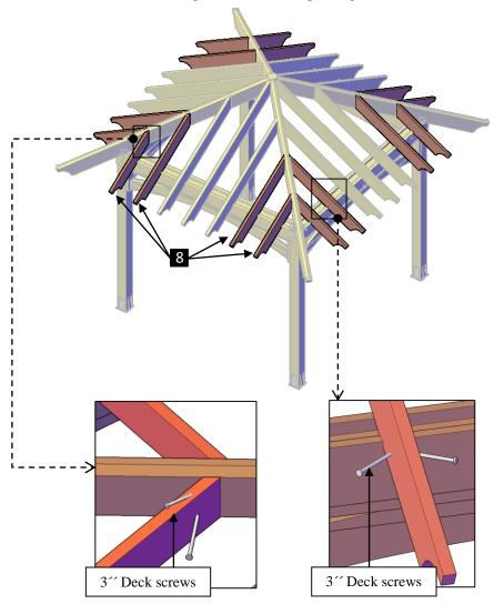
**Step 12:** Use 8" x 2 ½" deck screws (**L**) to attach the fascia boards (**9**) to the rafters, central rafters and diagonal rafters. Each part has a series of numbers that indicate where to attach the part with the corresponding number.
