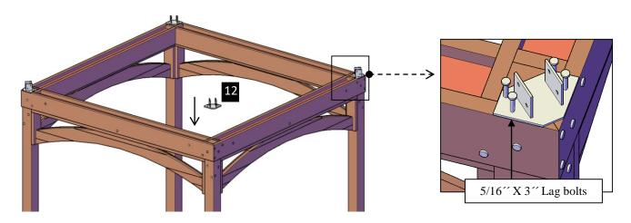
**Step 7:** Attach a diagonal rafter (7) to the second frame (5) with 3/8" x 6" lag bolts (C). After that, attach to its metal plaques (12) with 5/16" x 3 ½" bolts (H). Each part has a series of numbers that indicate where to attach the part with the corresponding number.
