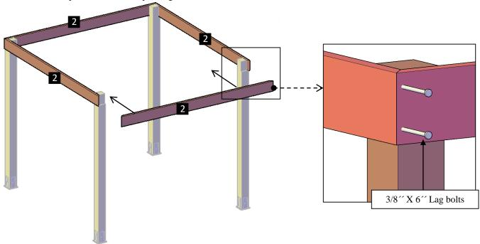
**Step 3:** Use 3/8" x 6" lag bolts (**C**) to attach the supports with in-between blocking (**3**) to the single supports. After that, use 3/8" x 10" lag bolts (**D**) to attach the supports with in between (**3**) to the posts and to the single supports. Each part has a series of numbers that indicate where to attach the part with the corresponding number.
