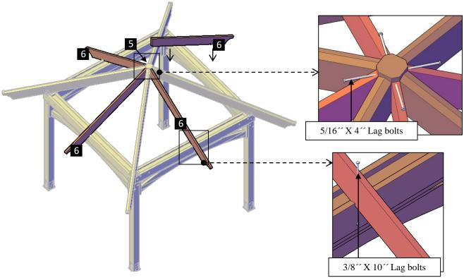
**Step 10:** Attach the rafters (8) to the diagonal rafters (7) with  $3^{\prime\prime\prime}$  deck screws (J) and to the single supports with  $3/8^{\prime\prime\prime}$  x  $10^{\prime\prime\prime}$  lag bolts (D). Each part has a series of numbers that indicate where to attach the part with the corresponding number.
