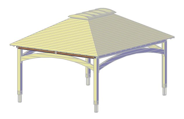
**Step 17:** Finally, use 3" deck screws (**DS1**) to attach the boots (**13**) to each post.
