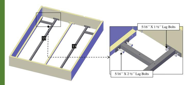
**Step 6:** Use 5/16" x 3" lag bolts (**F**) and 3" deck screws (**B**) to attach the top base to the bottom base, as shown below. Each part has a series of numbers that indicate where to attach the part with the corresponding number.
