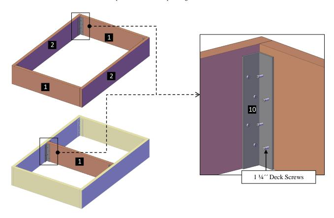
**Step 2:** To assemble the top base (3,4,5) use the angles (10) and  $1\frac{1}{4}$  deck screws (A), as shown below. Each part has a series of numbers that indicate where to attach the part with the corresponding number.
