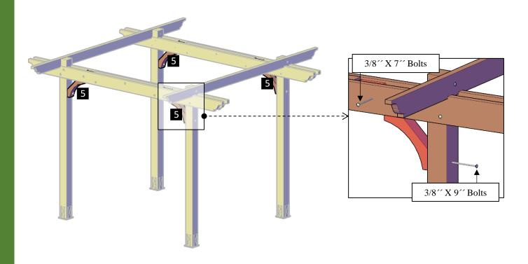
**Step 7:** Attach the secondary knee braces (6) to the posts with 3/8" x 9" bolts (F) and to the rafters with 3/8" x 5" bolts (C). Each part has a series of numbers that indicate where to attach the part with the corresponding number.
