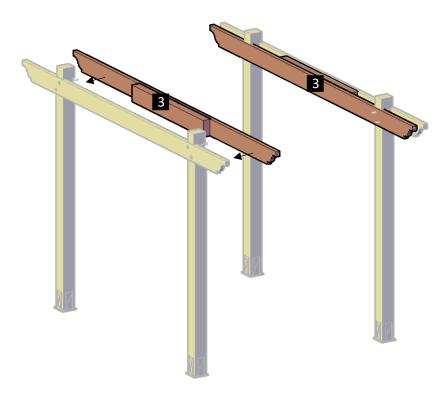
**Step 4:** Attach the single supports (2) to the supports with in-between blocking (3), use 3/8" X 7" bolts (C). The quantity of bolts depends on the length of the supports.
