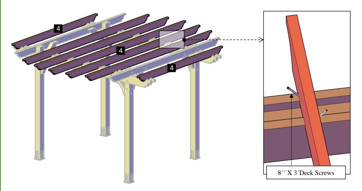
**Step 9:** Use 8" x 3" deck screws (**E**) to attach each slats (**7**) to the rafters. Each part has a series of numbers that indicate where to attach the part with the corresponding number.
