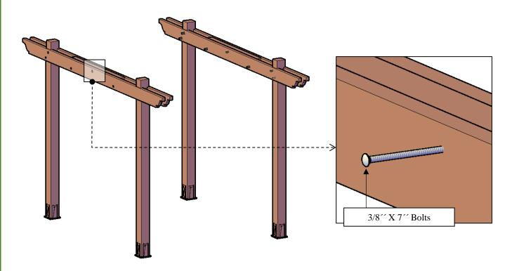
**Step 5:** Attach the perimeter rafters first (4) to the posts with 3/8 X 6 bolts (**D**) and to the supports with 8 x 3 deck screws (**E**). Each part has a series of numbers that indicate where to attach the part with the corresponding number.
