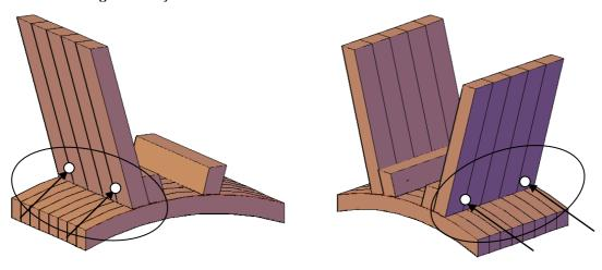
**Step 2**: Attach base support to both legs with 2 carriage bolts, washers and nuts per leg. Make sure that the numbers written next to the predrilled holes match.
