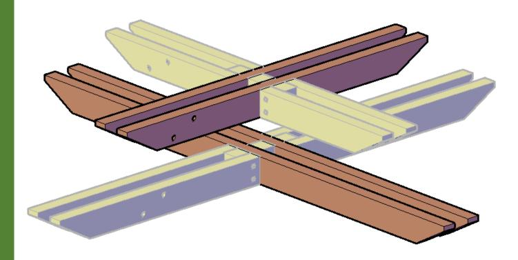
**Step 5:** Place the upper supports upside down. After that, attach the legs (6) to the upper supports with 3/8" X 9 ½" bolts (B). Each part has a series of numbers that indicate where to attach the part with the corresponding number.
