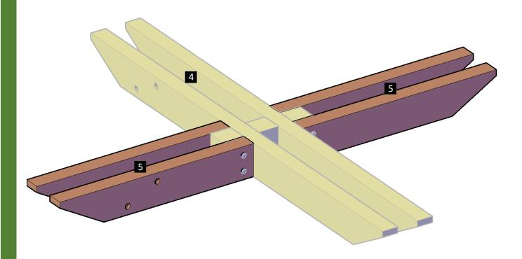
**Step 4:** Before attaching the legs to the supports make sure the long supports are not in the same direction. Each part has a series of numbers that indicate where to attach the part with the corresponding number.
