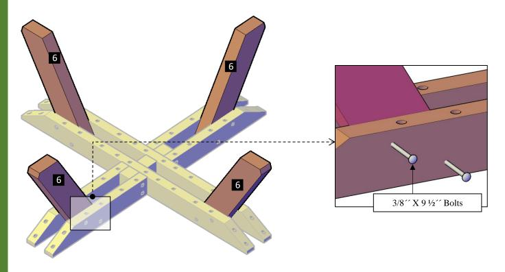
**Step 6:** Attach the lower supports (4,5) to the legs with 3/8" X 9  $\frac{1}{2}$ " bolts (B). Each part has a series of numbers that indicate where to attach the part with the corresponding number.
