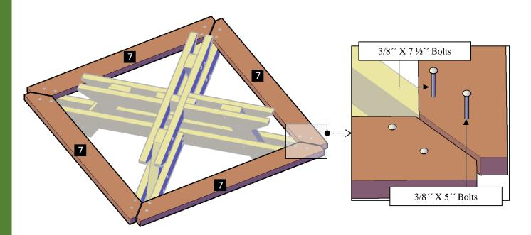
**Step 8:** Attach the tabletop boards (**8**) to the upper supports with 3/8  $\times$  X 8  $\frac{1}{2}$  bolts (**E**). The perimeter tabletop boards will be attached to the upper supports with 3/8  $\times$  X 7 bolts (**F**), and 3/8  $\times$  X 4  $\frac{1}{2}$  bolts (**G**). Each part has a series of numbers that indicate where to attach the part with the corresponding number.
