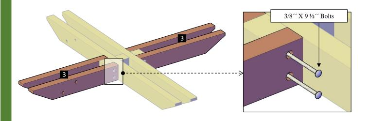
**Step 3:** To assemble the long and short lower supports (4,5), repeat the steps 1 and 2. Each part has a series of numbers that indicate where to attach the part with the corresponding number.
