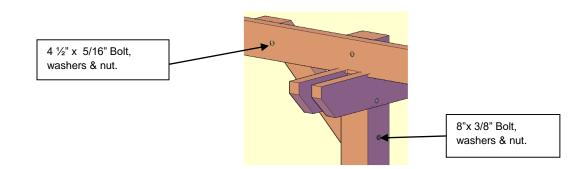
**Step 5.** Attach main knee brace to post & dual support beam with two bolts, washers & nuts. (Match numbers).Tap the bolt all the way into the wood to set it, then add a washer and nut and lightly tighten. *Repeat this step with the other main knee braces.*
