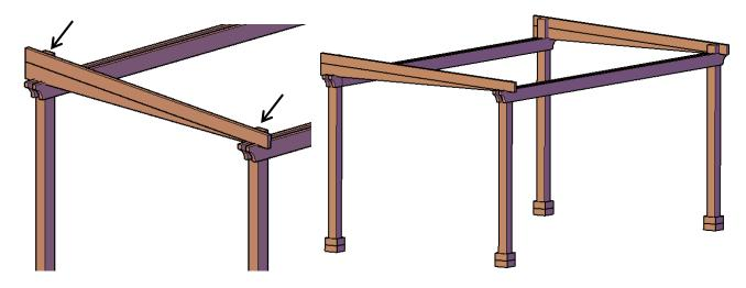
**Step 4.** Attach secondary knee brace to post & rafter with two bolts, washers & nuts. (Match numbers). Tap the bolt all the way into the wood to set it, then add a washer and nut and lightly tighten. *Repeat this step with the other end arch.*
