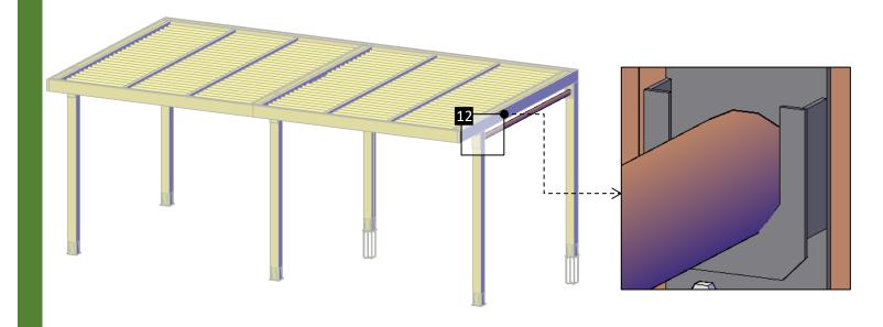
**Step 18:** Finally, attach the boots (15) to the posts with 3" deck screws (DS1).
