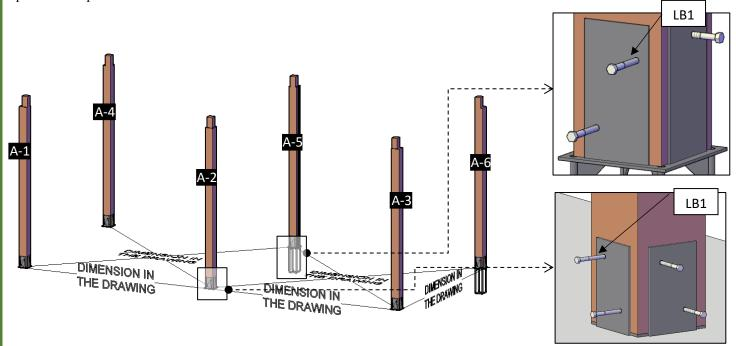
Step 2: Use 3/8" X 7 1/4" bolts (BL1) and 3/8" X 8" bolts (BL2) to attach the single Supports-B (3) to the posts (1). Check the marked on each support and place as drawings shown.
