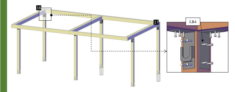
Step 12: Use 2" Deck Screws (DS2) to attach the L-plaques cover (14) to the posts and to the supports.
