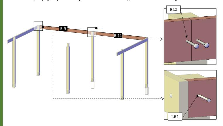
**Step 4:** Place the supports with in between blocking-A (5) into the post notches. Return to the bolts described in the step 3 and tighten fully. After that use 3/8" X 7 1/4" bolts (**BL1**) to attach the supports together. Check the marked numbers on each support with in-between blocking and place as drawings shown.
