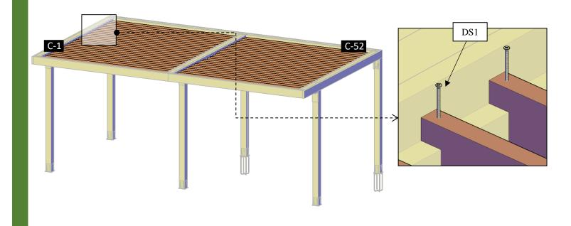
Step 15: Use 3" deck screws (DS1) to attach the slats (11) to the rafters (8). Check the marked on each slat and place as drawings shown.
