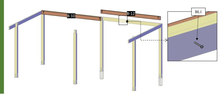
**Step 5:** Use 3/8" X 7 1/4" bolts (**BL1**) to attach the single Supports-C (**4**) to the posts (**1**). Check the marked on each support and place as drawings shown.
