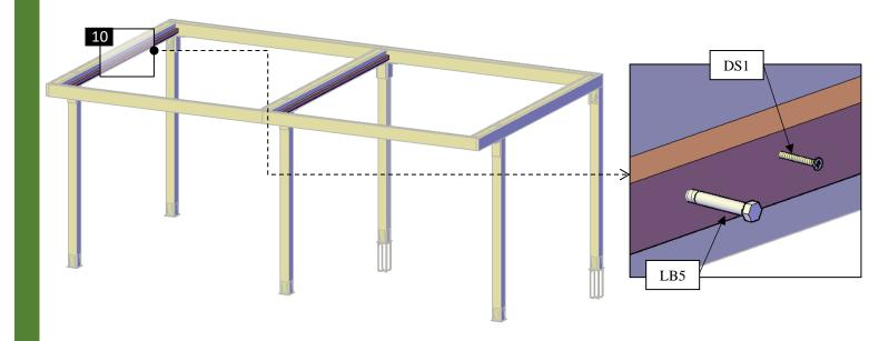
**Step 14:** Attach the rafters **(8)** to the Increase of rafters **(10)** with 3" deck screws **(DS1)**. Check the marked on each rafter and place as drawings shown (C-1 at C-52).
