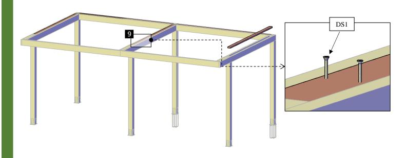
Step 11: Use 3/8" x 2 ½" lag bolts (LB4) to attach the L-Plaques (16) and curtain bases (17) to the posts and to the supports.
