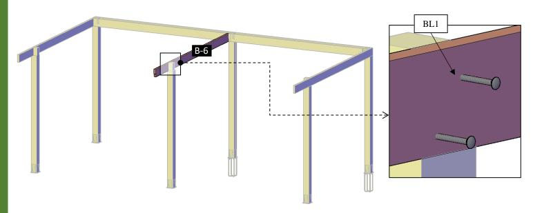
**Step 6:** Place the supports with in between blocking-B&C (**6, 7**) into the post notches. Return to the bolts described in the step 3 and tighten fully. After that use 3/8" X 7 ½" bolts (**BL1**) to attach the supports together. Check the marked numbers on each support with in-between blocking and place as drawings shown.
