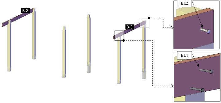
**Step 3:** Use 3/8" X 10" lag bolts (**LB2**) and 3/8" X 8" bolts (**BL2**) to attach the single Supports-A (**2**) to the posts (**1**). Check the marked on each support and place as drawings shown.
