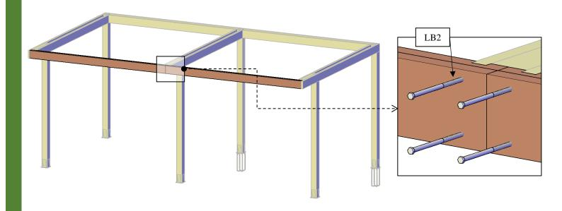
Step 10: Use 3" deck screws (DS1) to attach the in-between blocking cover (9) to the supports with in-between blocking.
