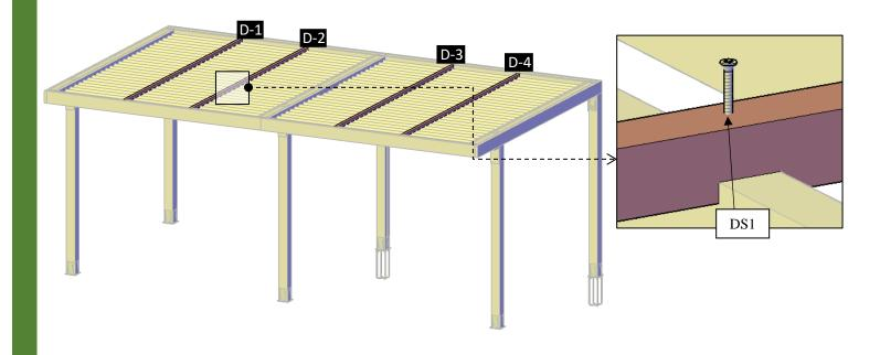
Step 16: Use 3/8" x 10 ½" bolts (BL3) to attach the ceiling fan base (13) to the rafters (8). Check the marked on each ceiling fan and place as drawings shown.
