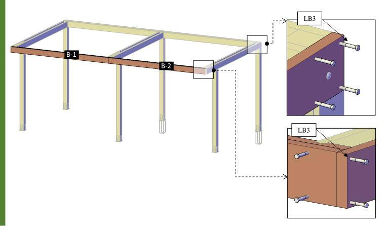
**Step 9:** Use 3/8" x 10" lag bolts (**LB2**) to attach the supports together. Check the marked numbers on each support and place as drawings shown.
