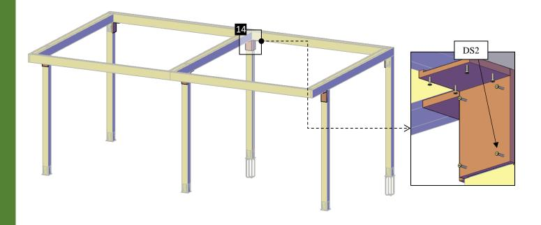
**Step 13:** Attach the increase of rafter (10) to the supports with 3" Deck Screws (**DS1**) and 3/8" x 5" lag bolts (**LB5**). Check the marked on each increase rafter and place as drawings shown.
