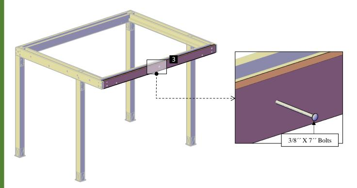
**Step 12:** Attach the in-between covers A&B (8,9) to the Supports A&B with in-between blocking, use 3'' deck screws (H). Each part has a series of numbers that indicate where to attach the part with the corresponding number.
