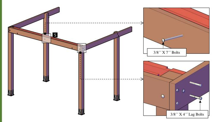
**Step 6:** Place the Supports-A with in-between blocking (4), into the post notches as shown and attach to the post with the single Supports-A bolts. Each part has a series of numbers that indicate where to attach the part with the corresponding number.
