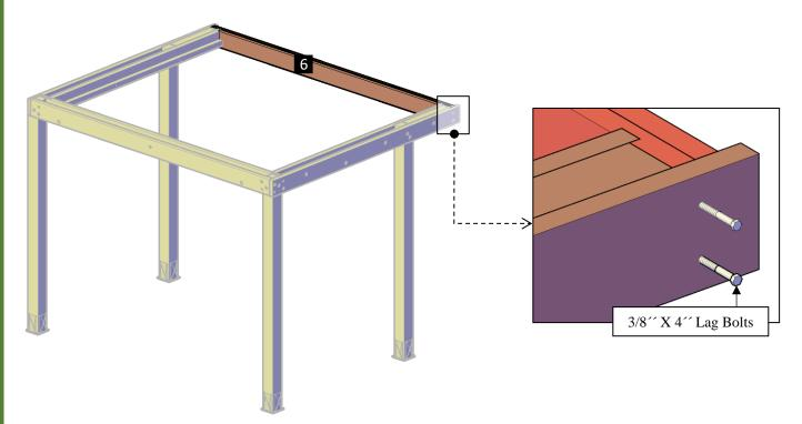
**Step 10:** Attach the Single Support-B (3) to the Single Supports-A with 3/8 x 4 lag bolts (F). After that, use 3/8 x 8 lag bolts (G) to attach to the Supports A&B with in between blocking. Each part has a series of numbers that indicate where to attach the part with the corresponding number.
