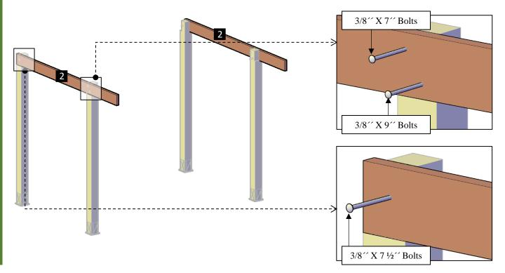
**Step 3:** Attach the Single Support-B (3) to the posts with 3/8 x 9 bolts (E). After that, use 3/8 x 4 lag bolts (F) to attach to the Single Supports-A. Each part has a series of numbers that indicate where to attach the part with the corresponding number.
