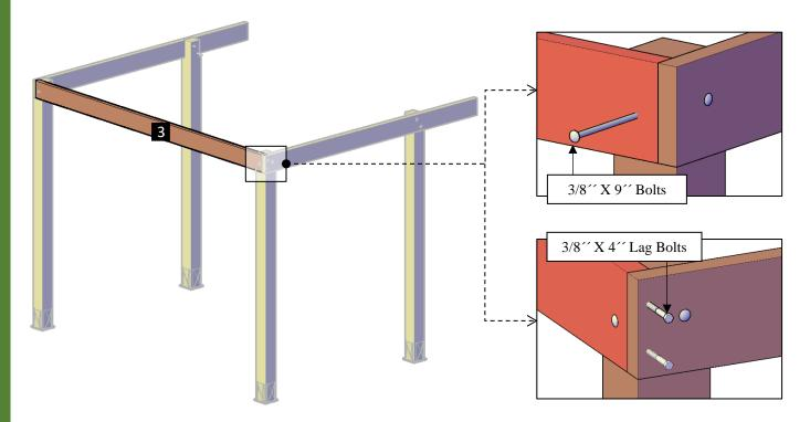
**Step 4:** Place the Support-B with in-between blocking (5), into the post notches as shown and attach to the post with the single Support-B bolts. Each part has a series of numbers that indicate where to attach the part with the corresponding number.
