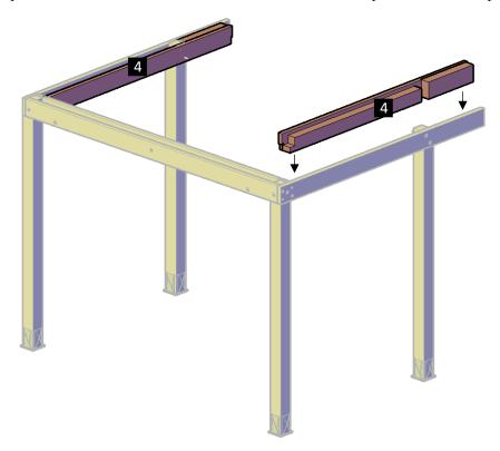
**Step 7:** Use 3/8<sup> $\prime'$ </sup> X 7<sup> $\prime'$ </sup> bolts (C) to attach the Single Supports-A to the Supports-A with in-between blocking (4). After that, attach the Supports-A with in-between blocking to the Supports-B, use 3/8<sup> $\prime''$ </sup> x 8<sup> $\prime''$ </sup> lag bolts (G).
