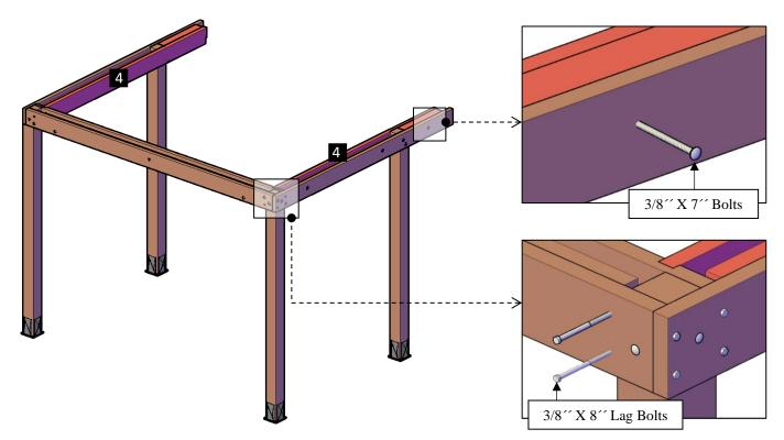
**Step 8:** Attach the lateral blockings (7) to the Supports-A with 3/8 x 9 bolts (E). Each part has a series of numbers that indicate where to attach the part with the corresponding number.
