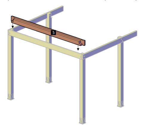
**Step 5:** Attach the Single Support-B to the Support-B with in-between blocking (5), use  $3/8^{\prime\prime} \times 7^{\prime\prime}$  bolts (C). After that, use  $3/8^{\prime\prime} \times 4^{\prime\prime}$  lag bolts (F) to attach the Support-B with in-between blocking to the Single Support-A.
