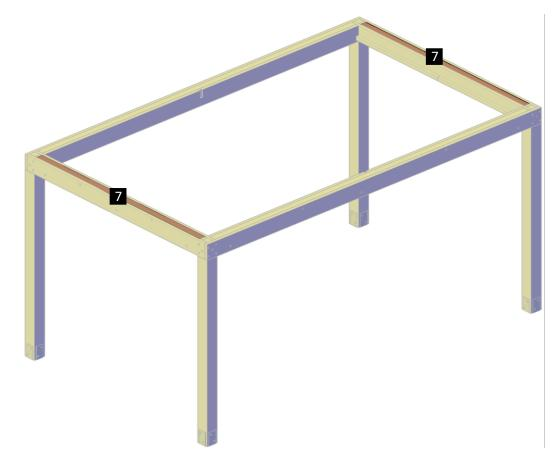
Step 9: Use 3/8 x 7 bolts (E) to attach the short in-between cover (7) to the short supports. Each part has a series of numbers that indicate where to attach the part with the corresponding number.
