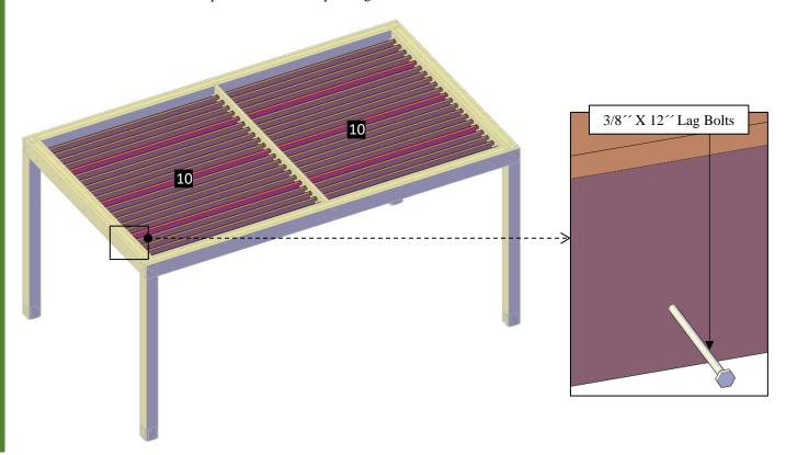
Step 15: Attach the slats (11) to the rafters with  $3^{\prime\prime}$  deck screws (L). Each part has a series of numbers that indicate where to attach the part with the corresponding number.
