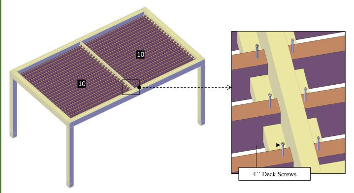
**Step 14:** Use 3/8 x 12 lag bolts (J) to attach the marked rafters (10) to the short supports. Each part has a series of numbers that indicate where to attach the part with the corresponding number.
