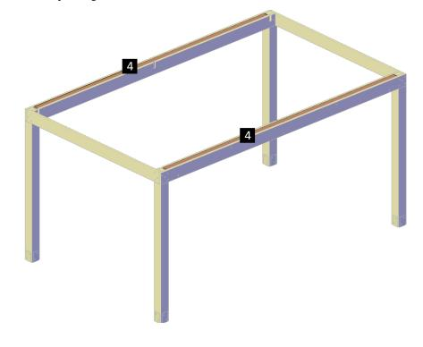
**Step 5:** Attach the long supports with in-between blocking (3) to the long single supports (2) and to the long in-between cover (4) with 3/8 x 7 bolts (E). Each part has a series of numbers that indicate where to attach the part with the corresponding number.
