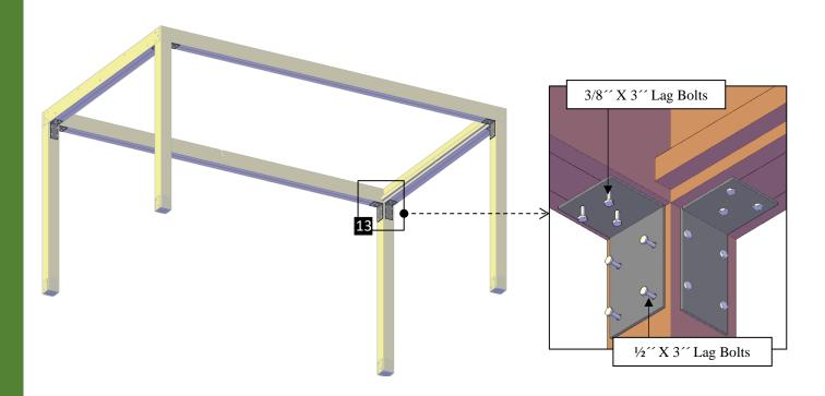
Step 11: Use 2<sup>--</sup> Deck Screws (I) to attach the angle covers (8) to the posts and to the supports. Each part has a series of numbers that indicate where to attach the part with the corresponding number.
