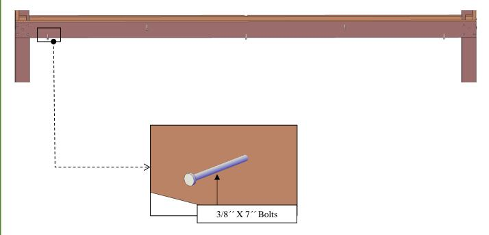
**Step 6:** Put up the short supports with in-between blocking (6) into the post notches and attach to the posts with the short single support bolt. After that, attach the short supports with in-between blocking (6) to the short single supports, used  $5/16'' \times 4''$  lag bolts (**D**). Each part has a series of numbers that indicate where to attach the part with the corresponding number.
