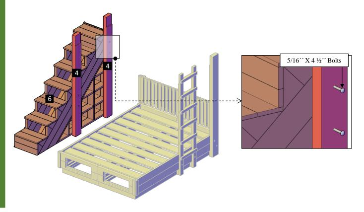
**Step 5:** Attach the top base (2) to the posts with 5/16" x 4" bolts (C). After that, use 5/16" x 3" bolts (A) to attach the top base to the ladder. Each part has a series of numbers that indicate where to attach the part with the corresponding number.
