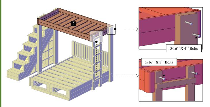
**Step 6:** Use 5/16 " x 5 ½" bolts (**E**) to attach the Knee Braces (**7**) to the posts. After that, attach to the top base with 5/16 " solts (**F**). Each part has a series of numbers that indicate where to attach the part with the corresponding number.
