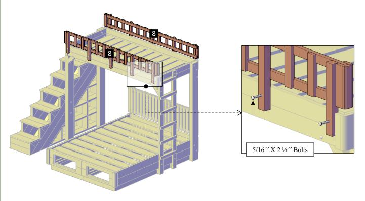
**Step 8:** Use 5/16 x  $3\frac{1}{2}$  bolts (**F**) to attach the short safety rails (**9**) to the top base. After that, attach to the long safety rails with  $2\frac{1}{2}$  deck screws (**B**). Each part has a series of numbers that indicate here to attach the part with the corresponding number.
