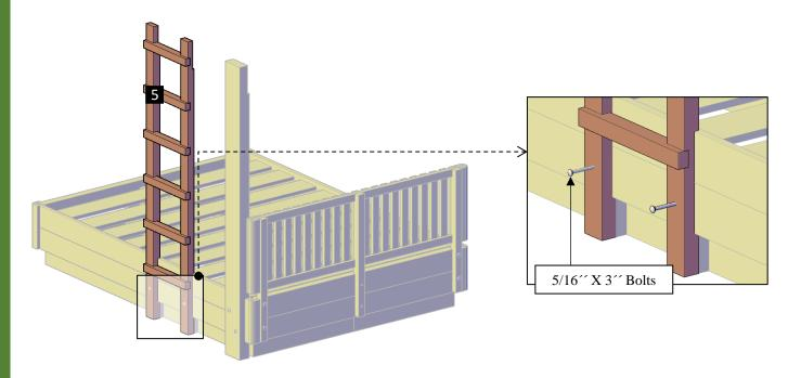
**Step 4:** Use  $5/16^{\prime\prime}$  x  $4\frac{1}{2}^{\prime\prime}$  bolts (**D**) to attach the posts (**4**) to the stairway (**6**). Each part has a series of numbers that indicate where to attach the part with the corresponding number.
