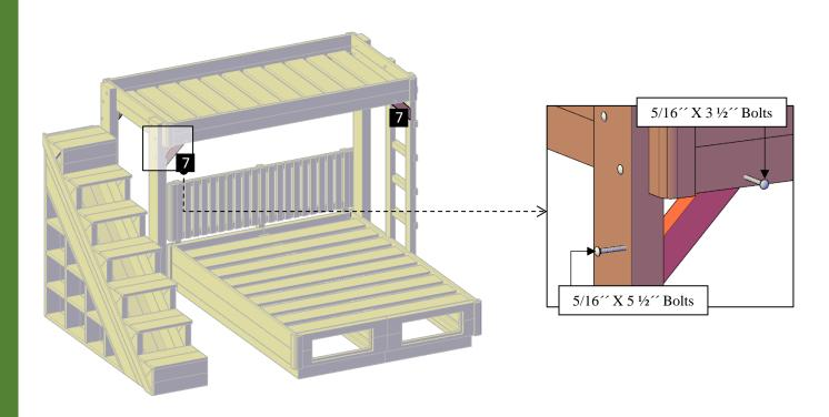
**Step 7:** Place the mattress on the top base. After that, attach the long safety rails (8) to the top base with 5/16" x 2 ½" bolts (G). Each part has a series of numbers that indicate here to attach the part with the corresponding number.
