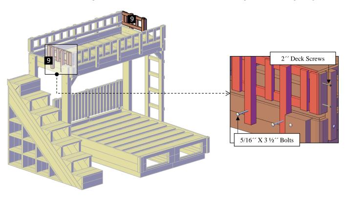
**Step 9:** Attach the stairway rails (10) to the stairway with 5/16 '' x 4 '' bolts (C) on the first step and 2  $\frac{1}{2}$  '' deck screws (B) on the rest. Each part has a series of numbers that indicate where to attach the part with the corresponding number.
