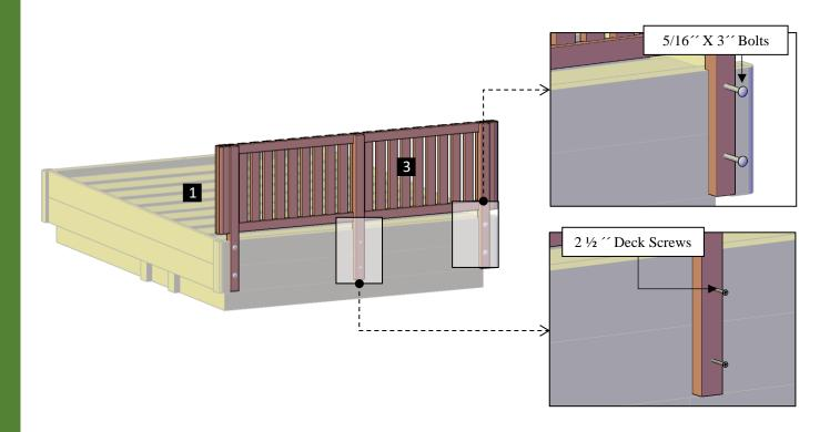
**Step 2:** Use 5/16" x 4" bolts **(C)** to one post **(4)** to the bottom base. Each part has a series of numbers that indicate where to attach the part with the corresponding number.
