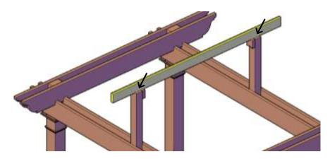
**Step 6.** Attach corner rafter to dual supports and center beam with galvanized deck screws (3" x #8).
