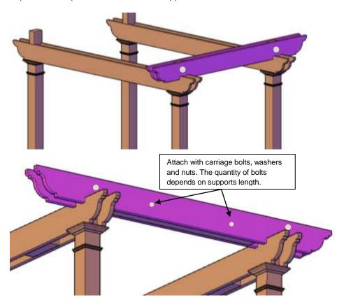
**Step 4.** Attach small post to dual supports with two bolts (8 "x 3/8") washers & nuts. (Match numbers). Tap the bolt all the way into the wood to set it, then add a washer and nut and lightly tighten. *Repeat this step with the other side.*
