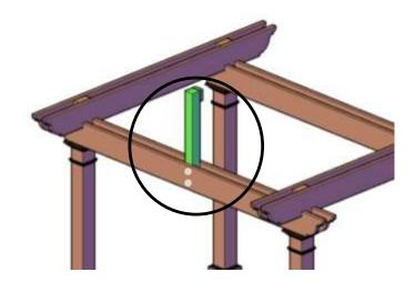
**Step 5.** Attach center beam to small posts with galvanized deck screws (3" x #8) at 45 degree angles to attach to the center beam. There are 8 screws used per center beam (4 per small post).
