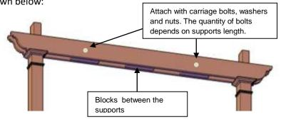
**Step 3.** Attach dual support beam in the other direction to posts with two bolts (8 "x 3/8") washers & nuts. (Match numbers). Tap the bolt all the way into the wood to set it, then add a washer and nut and lightly tighten. Repeat this step with the other dual support beam.
