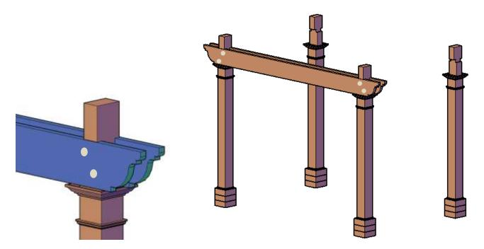
One the 2 supports have one large beam already attached or a few 18" pieces depending on size, this add support and strength to the structure. This beam must be in the interior of the support and bolted after you attach the supports to posts as shown below:
