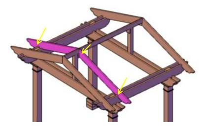
**Step 8.** Attach Tongue and groove boards to rafters with deck screws (1 5/8" x #8). The tongue and groove boards are all notched identically. The tongue and groove boards are notched to fit into each other. Place the center board first (the board with groove on one side and angle on the other) and then the rest for both sides.
