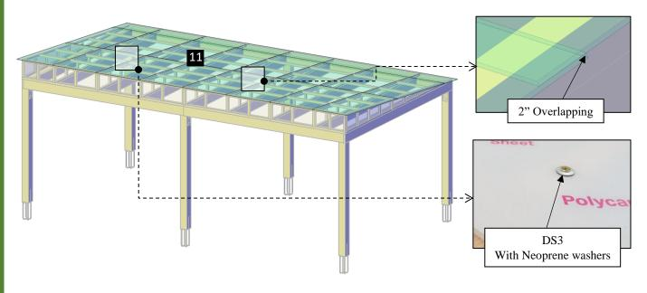
Step 14: Put exterior clear silicone and metallic tape 48mm x 50m on the polycarbonate (12) joins.
