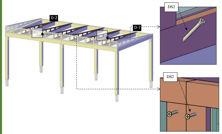
**Step 12:** Attach the reinforcement rain guard (10) to the rain guard (8) with  $2\frac{1}{2}$ " deck screws (**DS2**). check the marked numbers on each reinforcement rain guard and place as drawings shown (E-1 at E-18).
