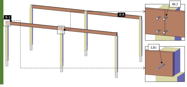
**Step 3:** Attach the supports to the supports with in-between blocking-A (3), use  $\frac{1}{2}$ " x 8  $\frac{3}{4}$ " bolts (**BL2**) with washer and nuts. After that, return to the bolts described in the step 2 and tighten fully. Check the marked numbers on each support with inbetween blocking and place as drawings shown.
