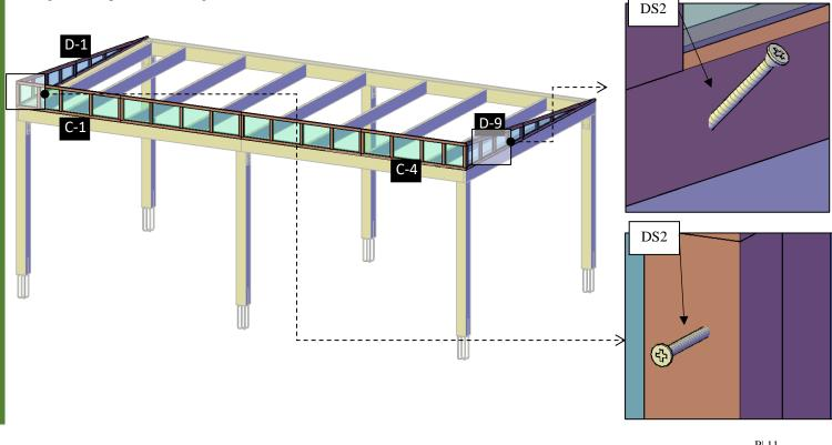
Step 9: Use 3/8 X 12" Lag Bolts (LB2) and 3"deck screws (DS1) to attach the central supports (6) to the supports. Check the marked number on each central supports and place as drawings shown.
