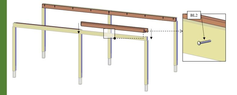
**Step 4:** Attach the single supports-B (4) to the posts with  $\frac{1}{2}$ " x 9" bolts (**BL3**) and use  $\frac{1}{2}$ " X 4" Lag Bolts (**LB2**) to attach the supports together. Check the marked numbers on each support and place as drawings shown.
