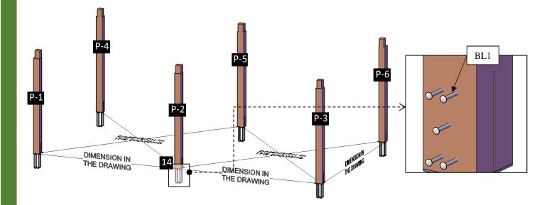
**Step 2:** Attach the single supports-A (2) to the corner posts with 3/8" x 12" lag bolts (**LB1**) and to the central posts with ½" x 8 <sup>3</sup>/4" bolts (**BL2**) with washer and nuts. Check the marked numbers on each support and place as drawings shown. *Note: Don't completely tighten yet the bolts and lag bolts– you will need the install the supports with in between blocking first. Note: drill the perimeter posts with the 1/2" x 12" bit.*
