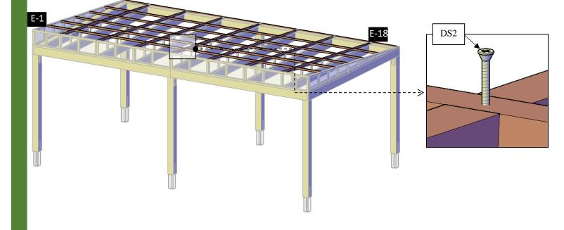
**Step 13:** Put the polycarbonate (11) from the bottom to the top, the overlapping between these it will be of 2". Attach to the center of the polycarbonate, use  $1\frac{1}{4}$ " deck screws (**DS3**) with neoprene washers. Each part has a series of numbers that indicate where to attach the part with the corresponding number.
