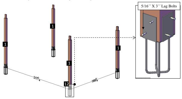
**Step 2:** Use 5/16 'X 4" Lag Bolts (**B**) and 3" Deck Screws (**C**) to attach the Single Supports-A (**2**) to the Central Supports (**4**). Each part has a series of numbers that indicate where to attach the part with the corresponding number.
