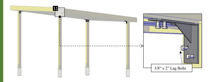
**Step 11:** Use 2 ½" Deck Screw (**G**) to attach the Tap L (**10**) to the posts and to the supports. Each part has a series of numbers that indicate where to attach the part with the corresponding number.
