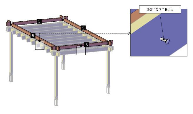
**Step 7:** Use 3/8" x 7" Bolts (**E**) and 3" Deck Screws (**C**) to attach the In-Between Blocking (**5**) to the Supports. After that. Cover the Deck Screws with taps. Each part has a series of numbers that indicate where to attach the part with the corresponding number.
