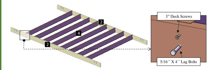
**Step 3:** Use 3" Deck Screws (**C**) to attach the Single Supports-A (**2**) to the Short Central Supports (**4**). Each part has a series of numbers that indicate where to attach the part with the corresponding number.
