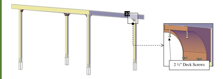
**Step 12:** Use 2" Deck Screws **(H)** to attach the Roof Boards **(8)** to the Supports. Each part has a series of numbers that indicate where to attach the part with the corresponding number.
