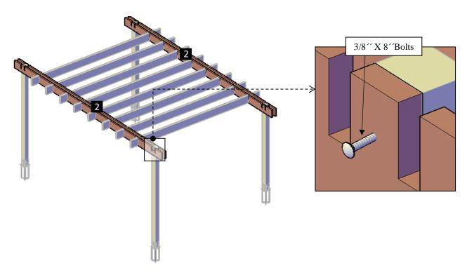
**Step 5:** Use 3/8" X 8" bolts (**D**) to attach the Single Supports-B (**3**) to the post (**1**). Each part has a series of numbers that indicate where to attach the part with the corresponding number.
