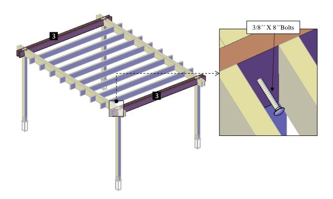
**Step 6:** Use 3/8" x 7" Bolts (E) to attach the In-Between Blocking (5) to the Supports. Each part has a series of numbers that indicate where to attach the part with the corresponding number.
