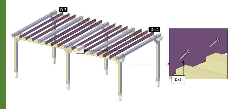
**Step 13:** Use 2" deck screws (**DS2**) to attach the roof board (9) to the rafters and supports. Check the marked numbers on each slat and place as drawings shown.
