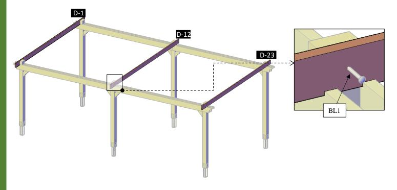
**Step 7:** Place the supports with in between blocking-B (**B**) into the post notches and attach the single supports-B (**4**) to the supports with in-between blocking (**3**), use 3/8" x 7 ¾" bolts (**BL1**) with washer and nuts. After that, return to the bolts described in the step 6 and tighten fully. Check the marked numbers on each support with in-between blocking and place as drawings shown.
