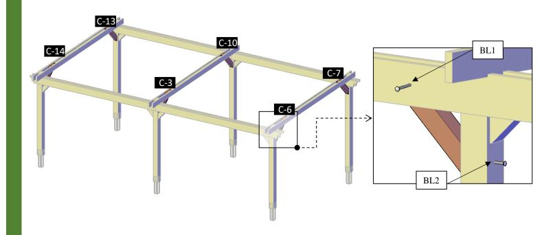
**Step 9:** Use 3/8" x 3" (**LB1**) to attach the metal plaques (**15**) to the supports.
