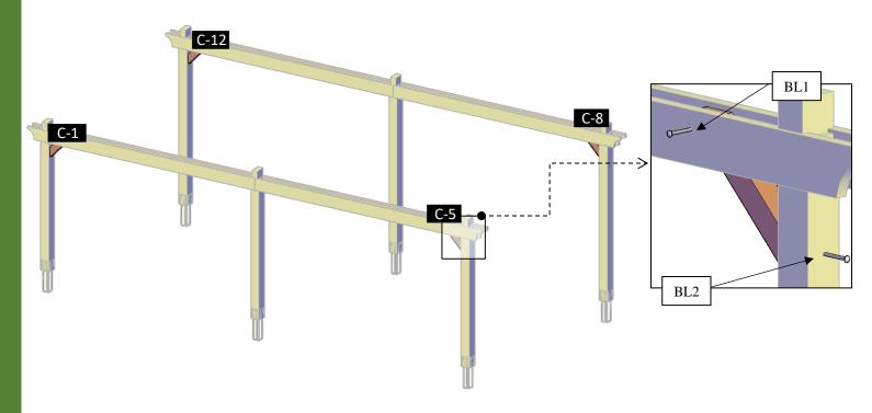
**Step 5:** Attach the central knee braces (7) to the supports with 3/8" x 7 3/4" bolts (**BL1**) and to the posts with 3/8" x 17" bolts (**BL3**) with washer and nuts. Check the marked numbers on each main knee braces and place as drawings shown.
