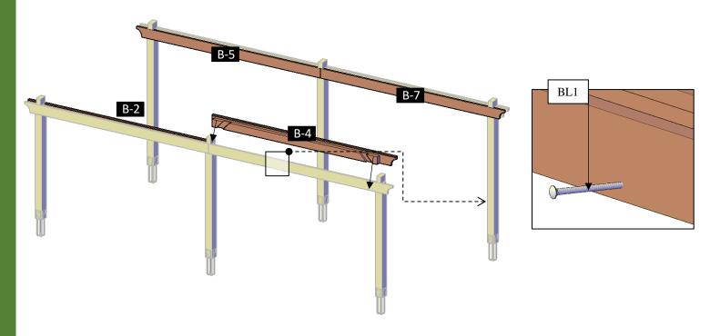
**Step 4:** Attach the main knee braces (7) to the supports with 3/8" x 7 3/4" bolts (**BL1**) and to the posts with 3/8" x 12" bolts (**BL2**) with washer and nuts. Check the marked numbers on each main knee braces and place as drawings shown.
