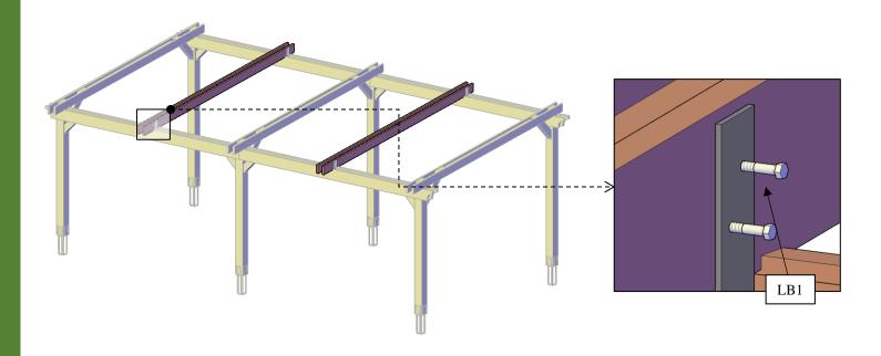
**Step 12:** Use 3" deck screws **(DS1)** to attach the rafters **(6)** to the supports. Check the marked numbers on each rafter and place as drawings shown (D-1 at D-21).
