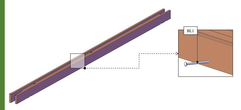
**Step 11:** Use 3/8" x 3" (**LB1**) to attach the supports to the metal plaques (15).
