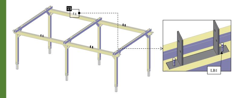
**Step 10:** use 3/8" x  $7\frac{3}{4}$ " bolts **(BL1)** with washer and nuts to attach the single supports-B **(4)** to the supports-B with in-between blocking-B **(5)**.
