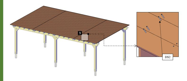
**Step 14:** Use 2" deck screws (**DS2**) to attach fascias (**10**) to the rafters and to the supports. Check the marked numbers on each fascia and place as drawings shown.
