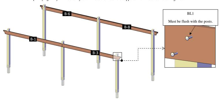
**Step 3:** Place the supports with in between blocking-A into the post notches and attach the single supports-A (2) to the supports with in-between blocking (3), use 3/8" x 7 3/4" bolts (BL1) with washer and nuts. After that, return to the bolts described in the step 2 and tighten fully. Check the marked numbers on each support with in-between blocking and place as drawings shown. *Note: put silicone in joints of the supports with in-between blocking.*
