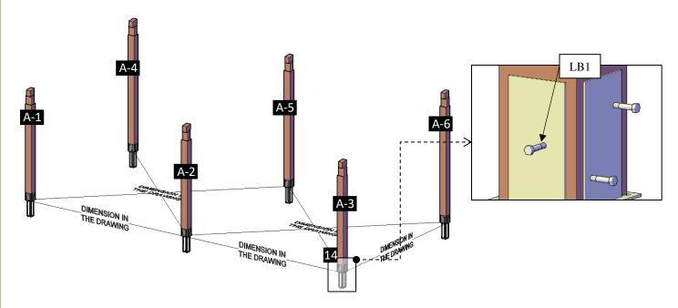
**Step 2:** Attach the single supports-A (2) to the posts with 3/8" x 7 <sup>3</sup>/<sub>4</sub>" bolts (**BL1**) with washer and nuts. Check the marked numbers on each support and place as drawings shown.
