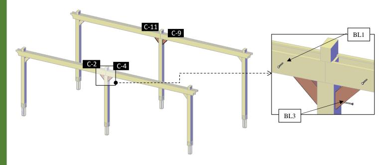
**Step 6:** Attach the single support-B (4) to the posts with 3/8" x 7 3/4" bolts (**BL1**) with washer and nuts. Check the marked numbers on each single support-B and place as drawings shown.
