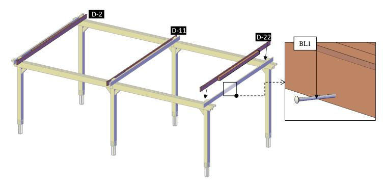
**Step 8:** Attach the secondary knee braces (8) to the rafters with 3/8" x  $7\sqrt[3]{4}$ " bolts (**BL1**) and to the posts with 3/8" x 12" bolts (**BL2**) with washer and nuts. Check the marked numbers on each secondary knee braces and place as drawings shown.
