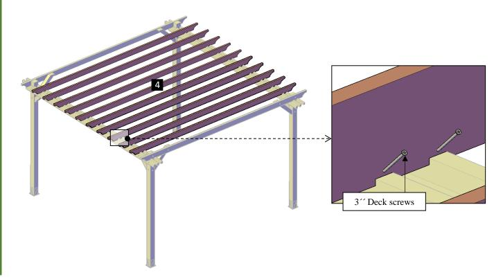
**Step 9:** Attach the Slats A&B (7,8) to the rafters with  $8'' \times 3''$  deck screws (F). Each part has a series of numbers that indicate where to attach the part with the corresponding number.
