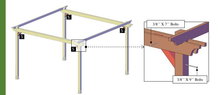
**Step 7:** Attach the Secondary knee braces (6) to the rafters with 5/16 x 5 bolts (G) and to the posts with 3/8 x 9 bolts (H). Each part has a series of numbers that indicate where to attach the part with the corresponding number.
