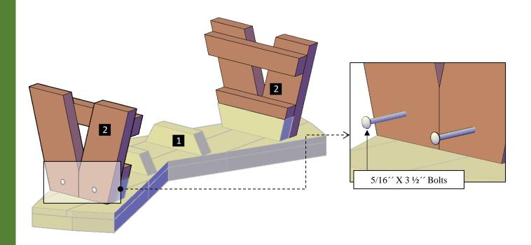
**Step 2:** Use 5/16" x 3 ½" bolts (**A**), washers and nuts to attach the diagonal supports (**3**) to the bench and to the seat. Each part has a series of numbers that indicate where to attach the part with the corresponding number.
