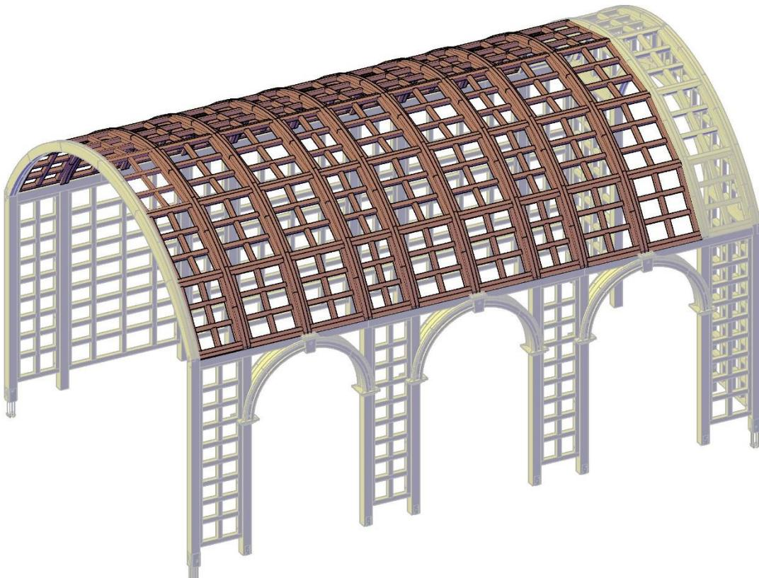
**Step 11:** Use 3'' deck screws □ (I) to attach the arc fascia (14) to the frontal arc.
