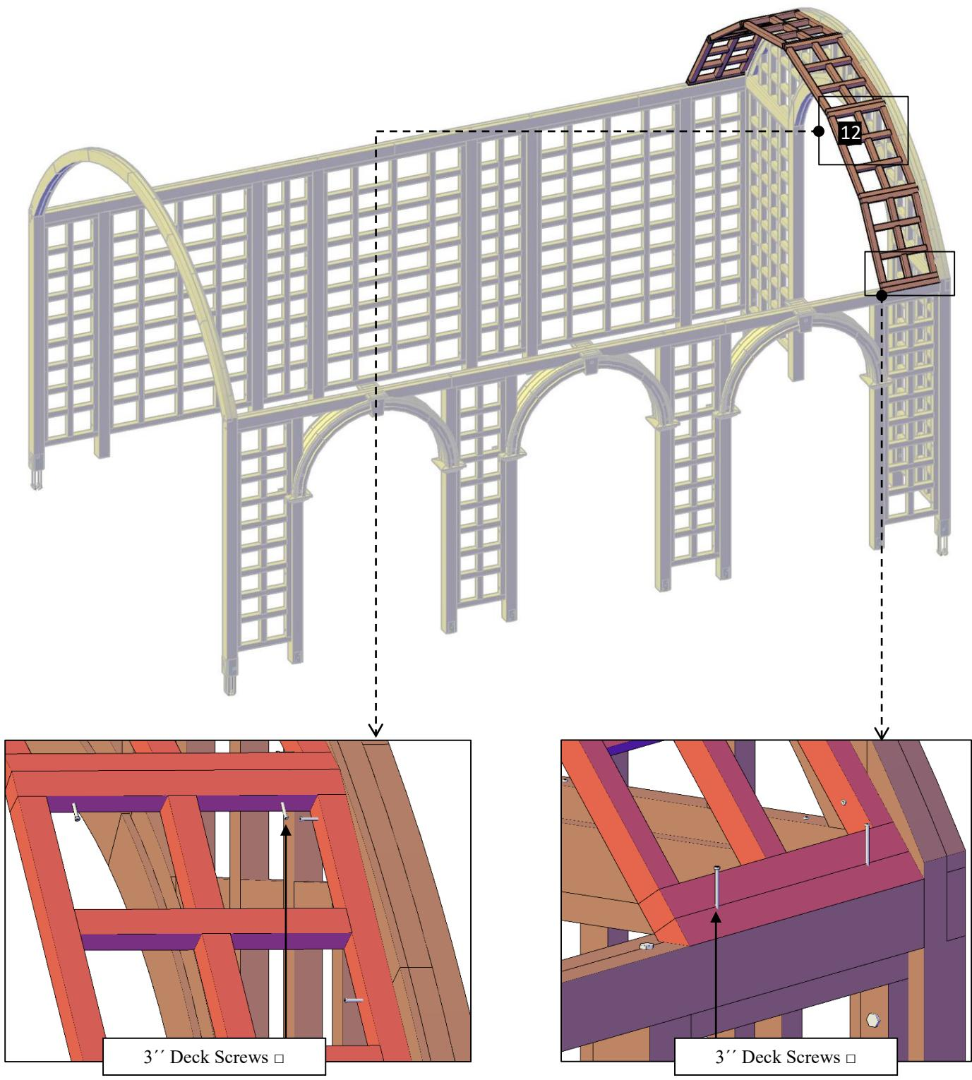
**Step 10.2:** Attach an arc (13) to the trellis with 3'' deck screws □ (I). After that, attach to the long supports with 4'' deck screws+ (J). Each part has a series of numbers that indicate where to attach the part with the corresponding number.
