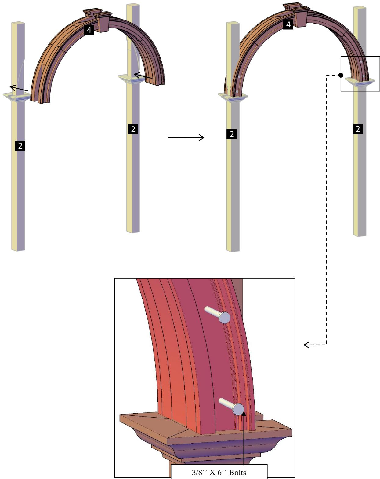
**Step 3:** Attach the wall trellis, the posts and the posts with arches, as shown below.
