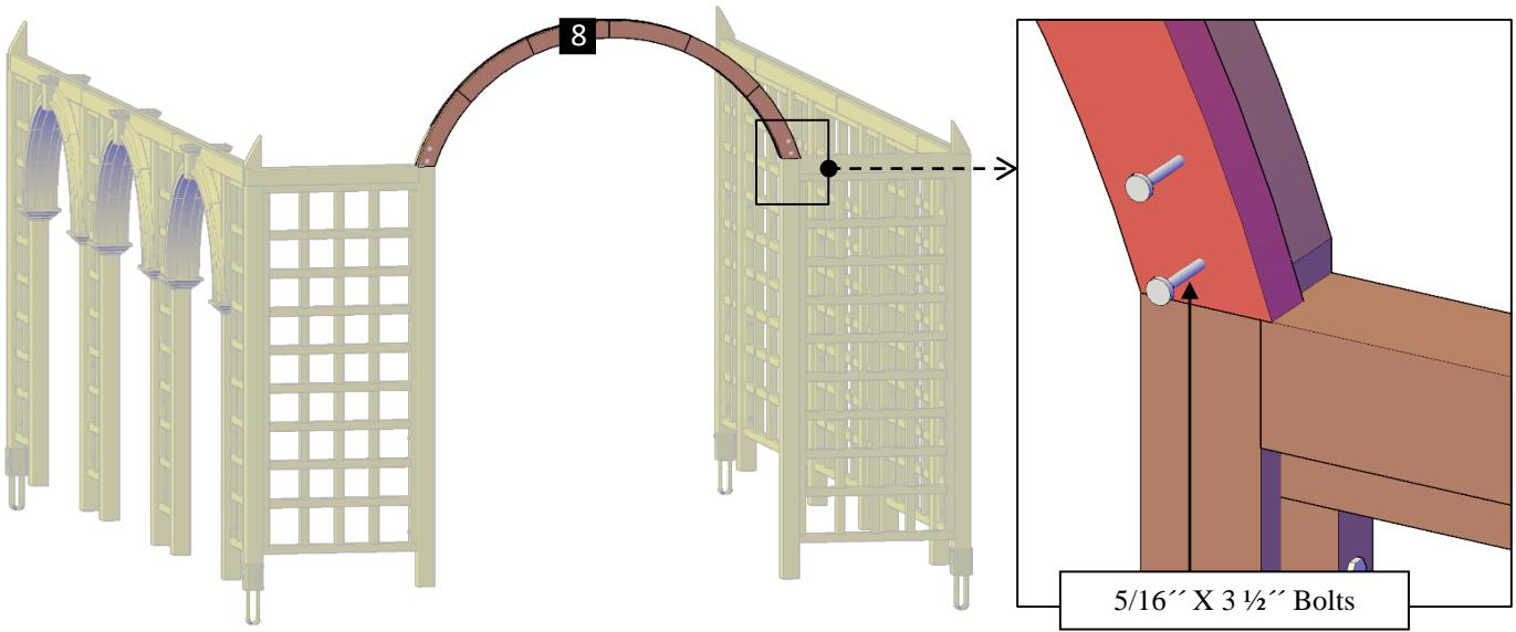
**Step 7:** Use 5/16" x 3 1/2" Bolts (**H**) to attach the perimeter arches (**9**) to the posts. Each part has a series of numbers that indicate where to attach the part with the corresponding number.
