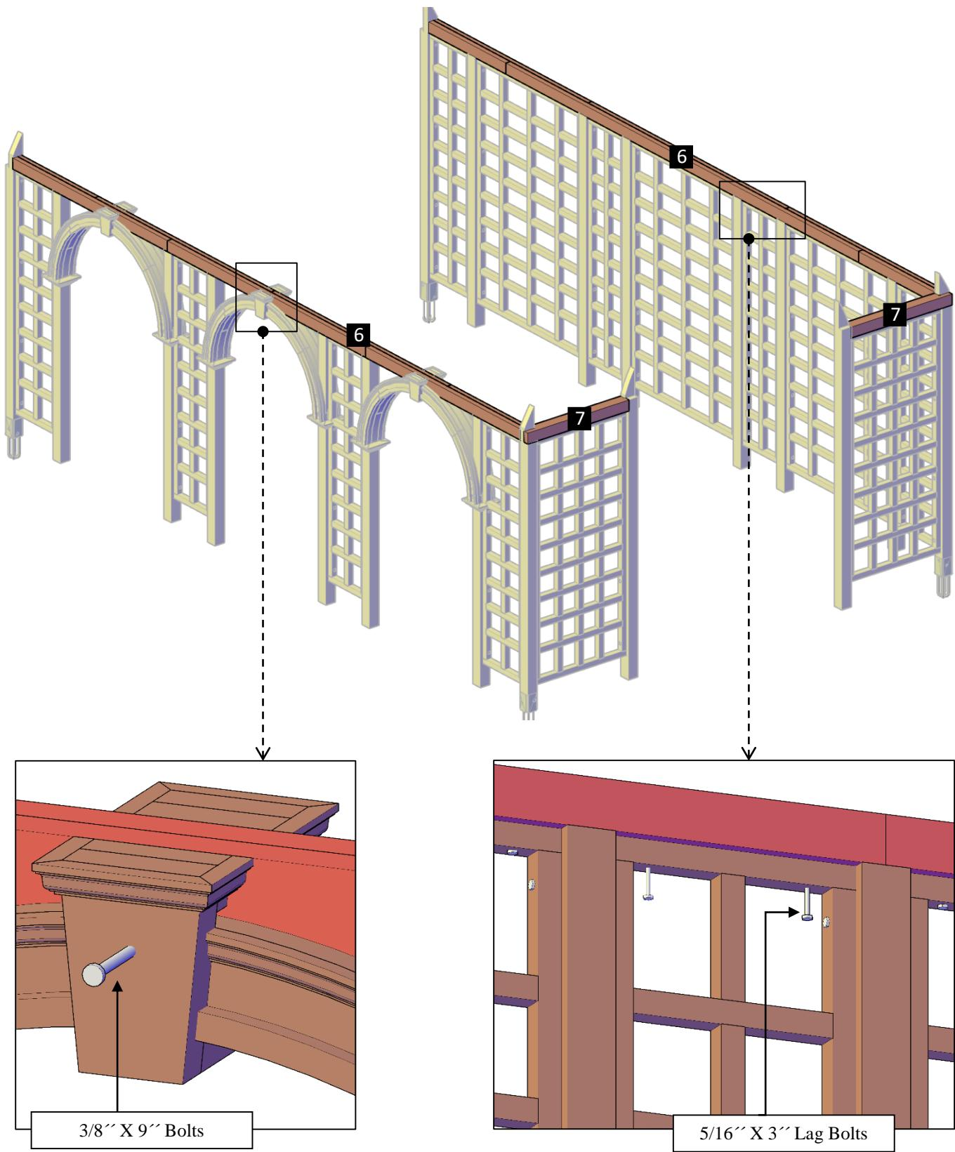
**Step 5:** Use  $3/8'' \times 8''$  lag bolts (**F**) and washers to attach the short supports (**7**) to the posts and to the long supports (**6**). After that, attach the long supports (**6**) to the posts with  $3/8'' \times 6''$  lag bolts (**G**) and  $3/8'' \times 8''$  Lag bolts (**F**) with Washers, as shown below. Each part has a series of numbers that indicate where to attach the part with the corresponding number.
