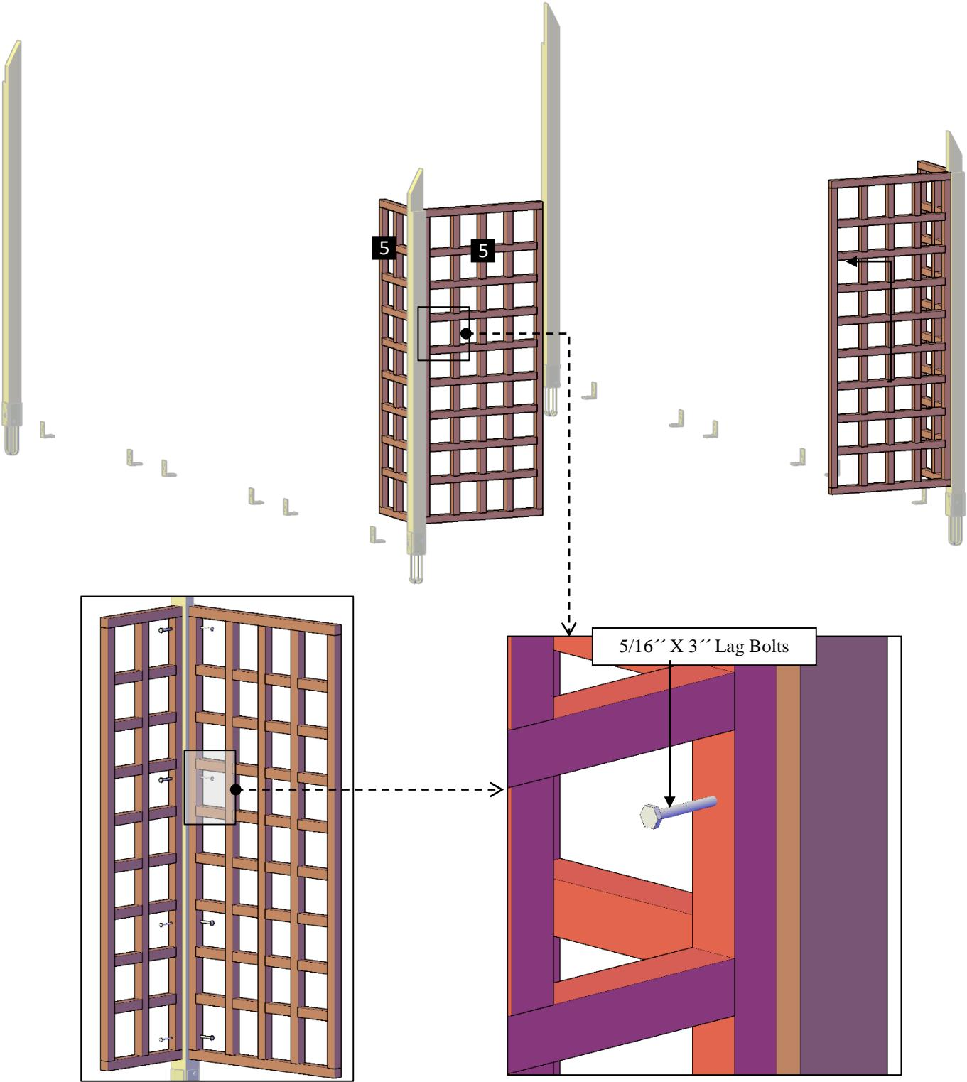
**Step 3.2:** Use 3'' deck screws + (D) to attach the posts to the angles. After that, attach the post to the trellis with 5/16'' x 3'' lag bolts (B) and washers. Each part has a series of numbers that indicate where to attach the part with the corresponding number.
