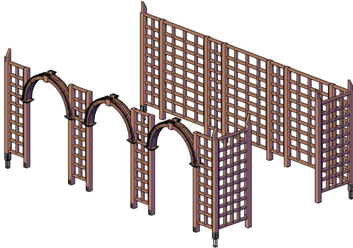
**Step 4:** Attach the long supports (6) and the short supports (7) to the trellis with 5/16" x 3" lag bolts with washers (B) and to the lateral arches with 3/8" x 9" bolts (E). Each part has a series of numbers that indicate where to attach the part with the corresponding number.
