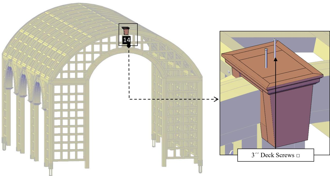
**Step 11:** Finally, use 3'' deck screws + (D) to attach the boots (15) to each posts.
