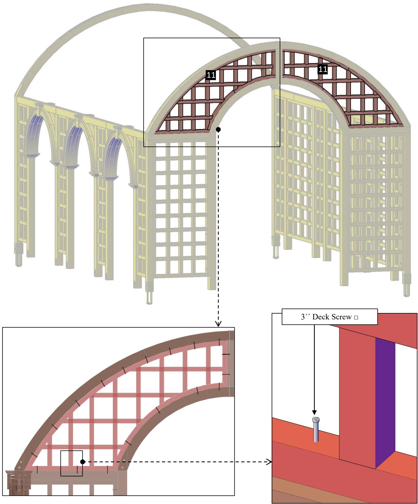
**Step 10:** Attach the arches and the trellis, as shown below.
