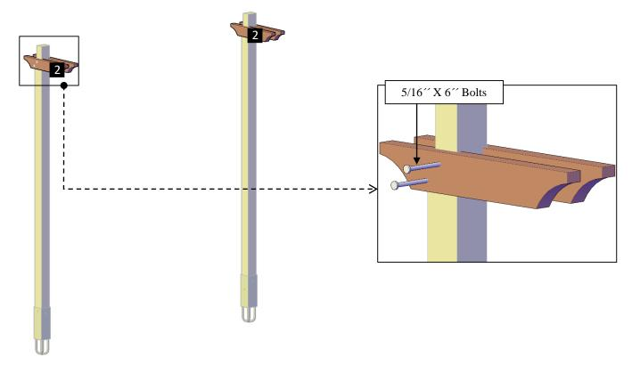
Step 3: Attach the knee braces (3) to the supports with  $5/16'' \ge 6''$  bolts (C) and to the post with  $3/8'' \ge 6 \frac{1}{2}''$  bolts (D). Each part has a series of numbers that indicate where to attach the part with the corresponding number.
