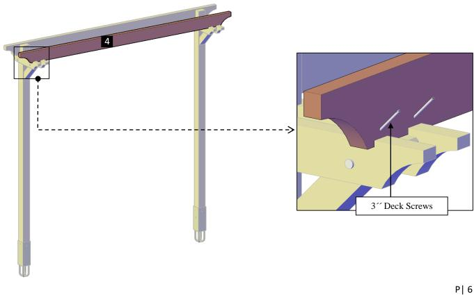
Step 6: Use 3<sup>---</sup> deck screws (F) to attach the slats (5) to the rafters. Each part has a series of numbers that indicate where to attach the part with the corresponding number.
