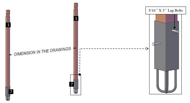
Step 2: Attach the supports (2) to the posts with 5/16" x 6" bolts (C). Each part has a series of numbers that indicate where to attach the part with the corresponding number.
