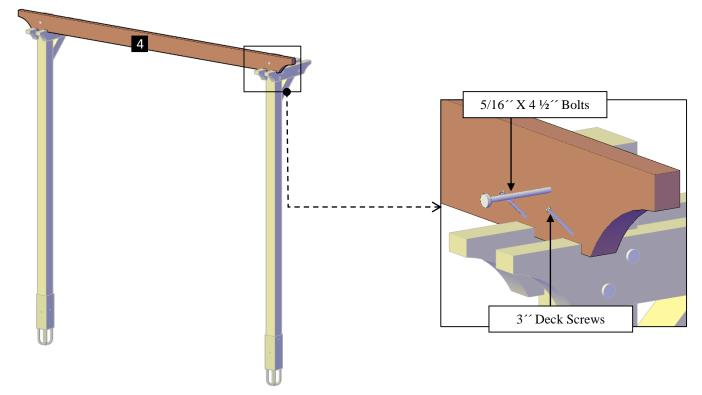
Step 5: Attach the other rafter (4) to the supports with 3" deck screws (F). Each part has a series of numbers that indicate where to attach the part with the corresponding number.
