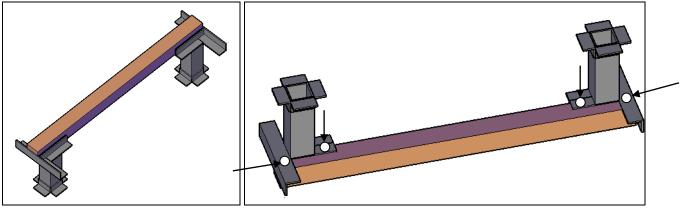
**Step 2:** Attach the rest of the boards to the legs with bolts (3"x 5/16") as shown below.
