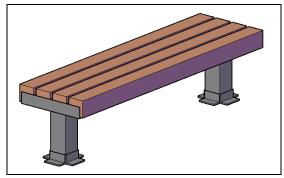
**Step 3:** The metal framing can be ordered as shown to bury underground with concrete 18" deep or the bottom can be bolted to the ground in the alternative method shown with anchor bolts into an existing concrete floor.
