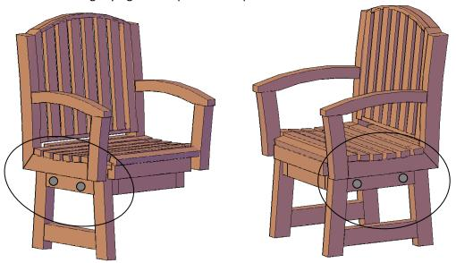
**STEP 4:** Attach the leg support to the leg assembly left, with two bolts (3  $\frac{1}{2}$ " x 5/16"), washers & nuts (Match up the numbers to attach the two parts together). Tap the bolt all the way into the wood to set it. Then add a washer and nut and lightly tighten. Repeat this step with the other side.
