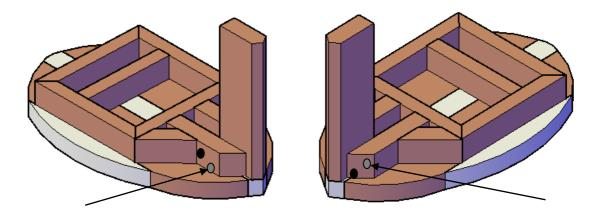
**Step 2:** Attach back legs to tabletop with 2 carriage bolts (5" x 5/16"), washers and nuts per leg.
