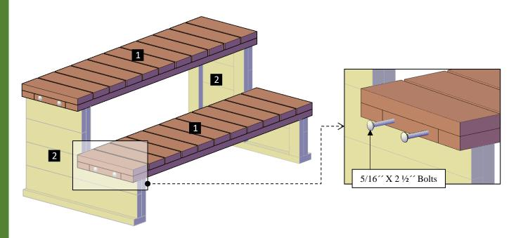
**Step 2:** Attach the central leg (3) to the steps, use 5/16 x  $2\frac{1}{2}$  bolts (A) with washers (C) & nuts (D). Each part has a series of numbers that indicate where to attach the part with the corresponding number.
